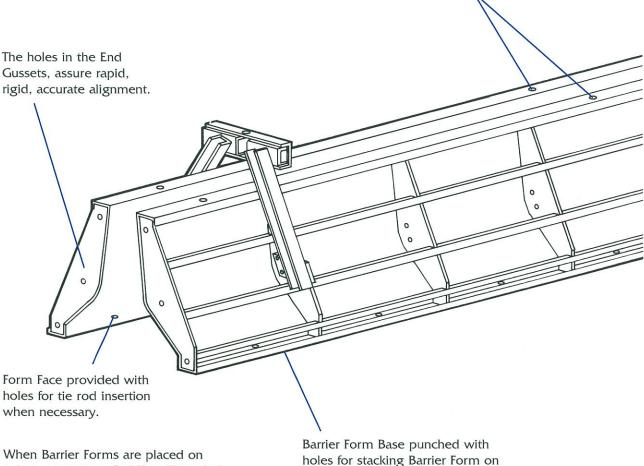
existing concrete, Coil Ties, Threaded Snap Rods and Nuts prevent forms from floating by tying down to Barrier Top Spacers or Yokes.
