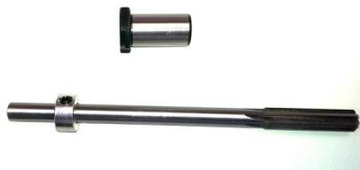
If you have Spacer Rings and/or Flange Ring, insert 1/2" bushing and use Reamer to enlarge through holes in Spacer Rings and/or Flange Ring-ONLY.
