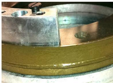
Position drill bushing over broken bolt
