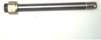
Assemble Long Installation Tool using 3/8" -16 x 5 1/2" Bolt
