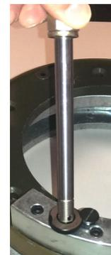
Insert 1/2" bushing into bushing block
