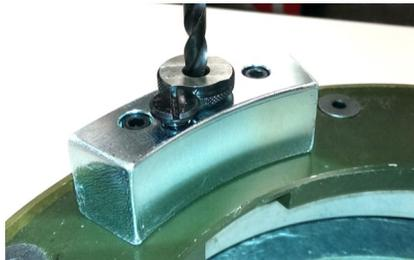
Use 15/32" drill bit, drill hole in top flange
