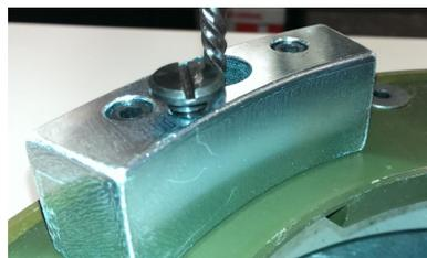
Remove 5/32" bushing, using reverse
