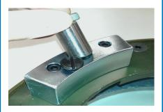
Insert 15/32" bushing into bushing block Apply liberal amount of tapping fluid
