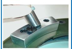
Insert 5/32" bushing into bushing block
