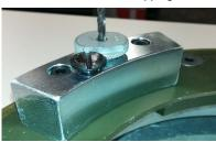
Use 5/32" drill to core our center of bolt (slow to medium drill speed preferred)
