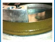
Position drill bushing over broken bolt and attach to light base using provided flat head bolts
