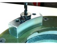
Use 5/16" drill and drill out remainder of broken bolt, being sure to drill all the way through top flange to be sure bolt is completely removed.
