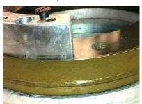
Position drill bushing over broken bolt and attach to light base using provided flat head bolts Note: (If applicable)
