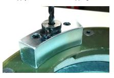
Use 15/32" drill bit, drill hole in top flange Drill through spacer rings if applicable If you do not have any Spacer Rings and/or Flange Rings, go to step #6
