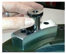
Insert 5/16" bushing into bushing block
